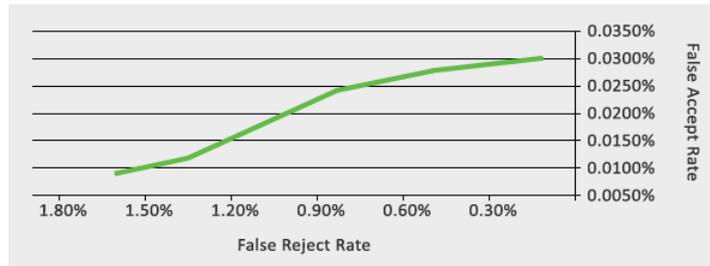
The graph indicates the ratio between the percentages of false reject (no-detection) to false accept (false detection) rates. The percentages of false accept are three cases out of 10,000 (3/10,000) when the false reject are at two cases out of 1,000 (2/1,000). When higher security is set and the percentages of false accept are one case out of 10,000 (1/10,000), the false reject rate will provide 15 cases out of 1,000 (15/1,000).
