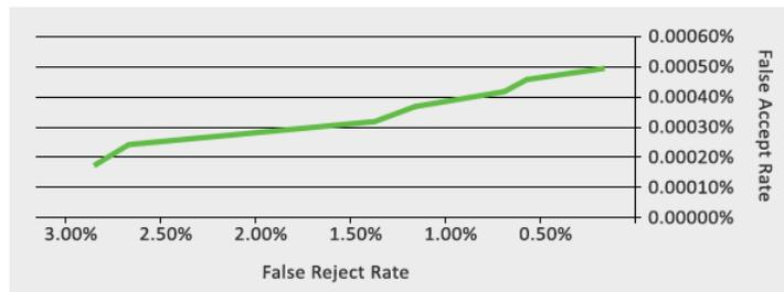
The graph indicates the ratio between the percentages of false reject (no-detection) to false accept (false detection) rates. The percentages of false accept are five cases out of 1,000,000 (5/1,000,000) when the false reject are at two cases out of 1,000 (2/1,000). When higher security is set and the percentages of false accept are two cases out of 1,000,000 (2/1,000,000) the false reject rate will provide 28 cases out of 1,000 (28/1,000).
